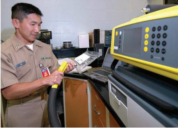
**Figure 3-6.** An industrial hygiene officer assigned to Navy Environmental and Preventative Medicine Unit Six (NEP-MU-6) tests an air sample for contaminants. US Navy photo by Journalist 2nd Class Ryan C. McGinley. Reproduced from: <http://www.navy.mil/management/photoadb/photos/060207-N-3019M-003.jpg>.
